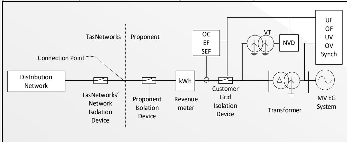
**Figure 2: Example of TasNetworks communications based anti-islanding inter-trip protection scheme.**
