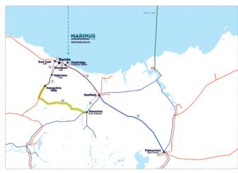
Between Staverton and Hampshire Hills a new double circuit 220 kV transmission line is proposed to be built within a predominantly new 90 metre wide easement.
