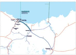
A new 220 kV double circuit transmission line is proposed to be built within the existing easement to replace the existing 220 kV single circuit line.
