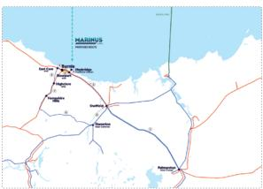
From Minna Road, Stowport to Burnie the existing single circuit flat spacer transmission infrastructure will be replaced with a new double circuit 220 kV transmission line.
