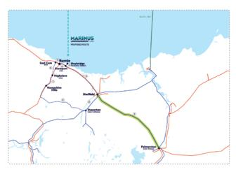
Between Palmerston and Sheffield a new double circuit 220 kV transmission line is proposed to be constructed adjacent to the existing single circuit 220 kV transmission line on the northeast side. This would require widening the existing easement by approximately 20 metres.
