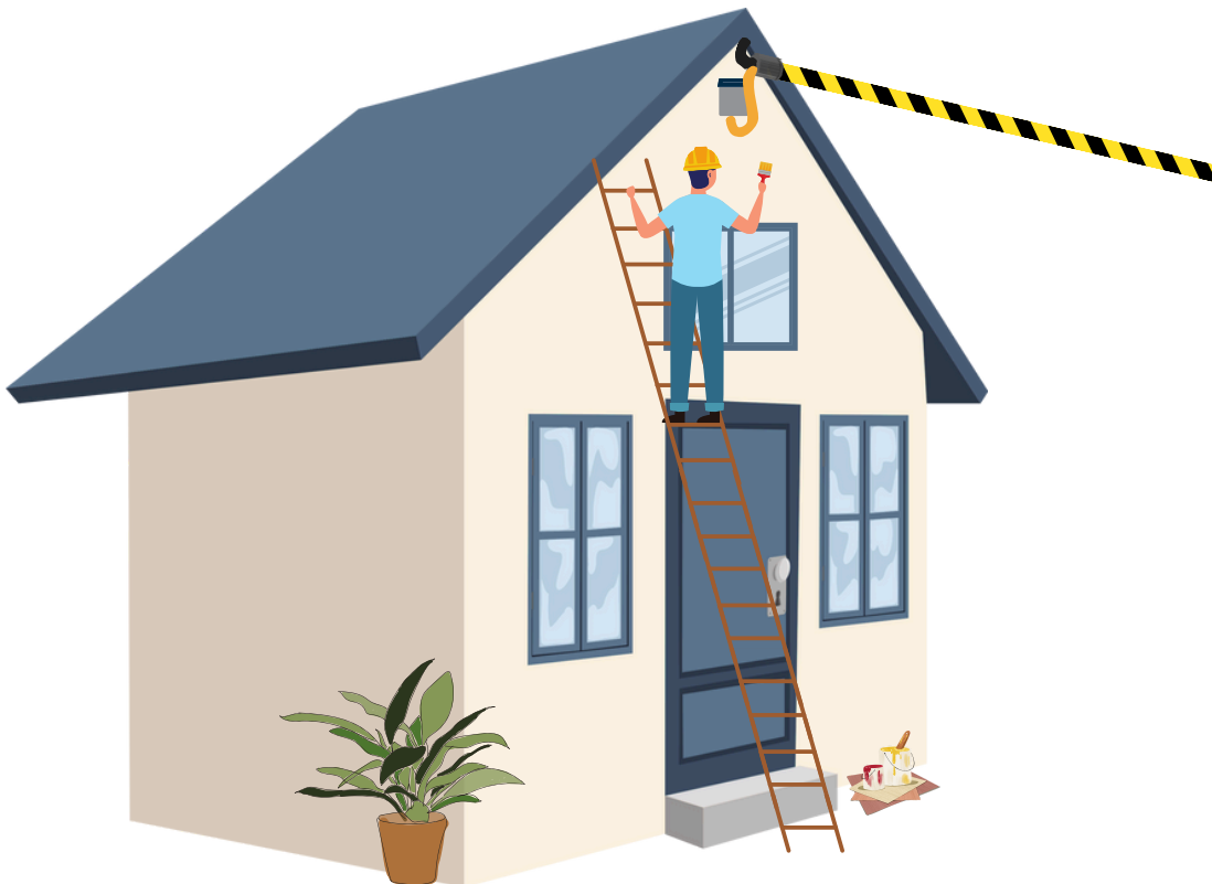
Figure 5: Workers or tools may come as close as they need to the insulated line but are not allowed to make contact.
