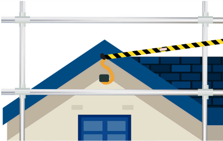
Figure 4: Where SADs cannot be maintained, insulated coverings like tiger tails can be used to protect against accidental contact.
