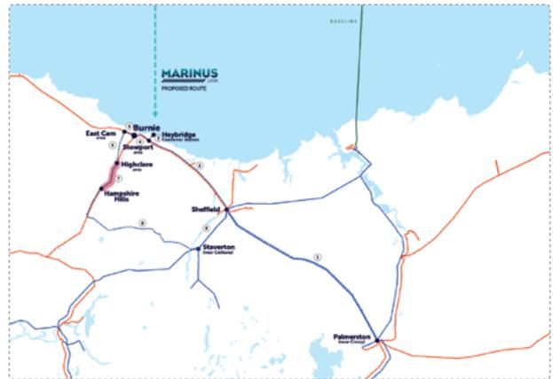
Between Highclere and Hampshire Hills a new double circuit 220 kV transmission line is proposed. Only one transmission line will be constructed initially, but there is provision for a second transmission line if required.
