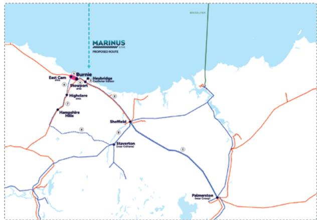
Between Burnie and East Cam, a new transmission line will be constructed next to the existing one, on the southern side, which will require the easement to be widened by 20 metres.
