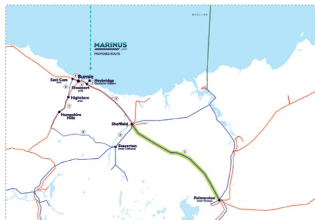
Between Palmerston and Sheffield a new double circuit 220 kV transmission line is proposed to be constructed adjacent to the existing single circuit 220 kV transmission line on the northeast side. This would require widening the existing easement by approximately 20 metres.
