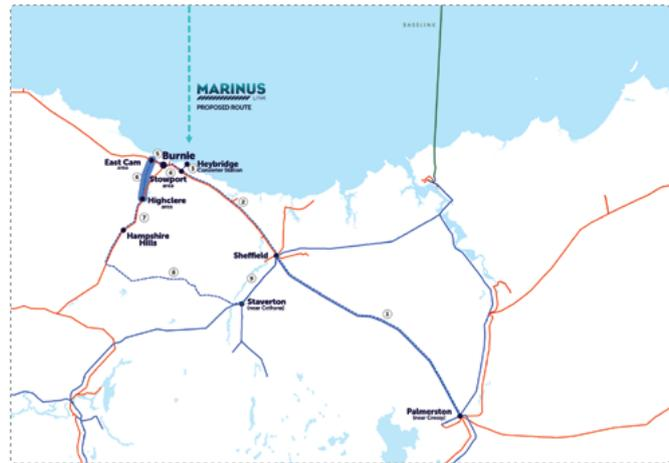
Between East Cam and Highclere a new double circuit 220 kV transmission line will be required in a new 90 metre wide easement. Only one transmission line will be constructed initially, but there is provision for a second transmission line to cater for future customer needs.
