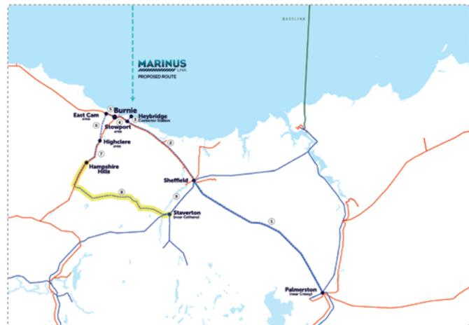
Between Staverton and Hampshire Hills a new double circuit 220 kV transmission line is proposed to be built within a predominantly new 90 metre wide easement.
