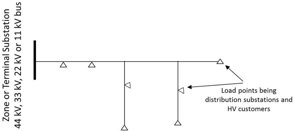
The standard methodology to calculate the loss component for the High Voltage Distribution Network is:
