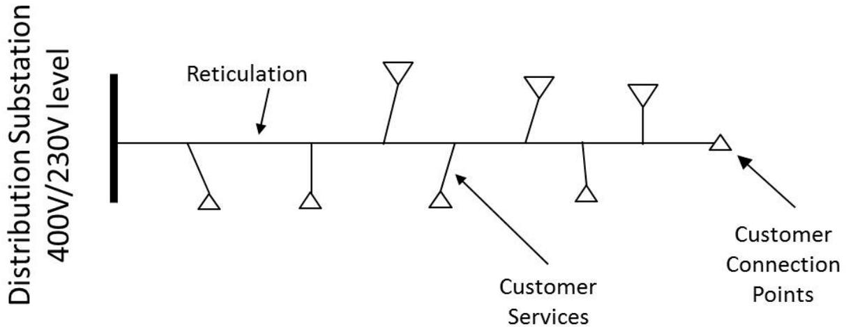
The standard methodology to calculate the loss component for the Low Voltage reticulation is:
