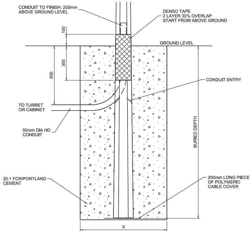
**HOLE DIAMETER 'X' WITH 20:1 FCR/CEMENT BACKFILL**
