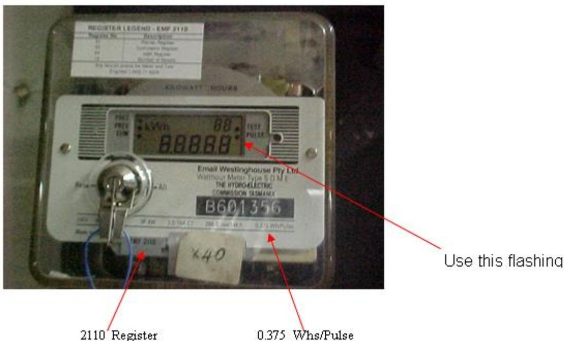
But  $1000/0.375 = 2666.66'$  as the test constant. Using this value gives an accuracy result of -99% (test set running too slow). So, we need to halve  $2666.66' = 1333.33'$  as the test constant. This gave an accuracy figure of 44.68% (on the right track but still incorrect).
