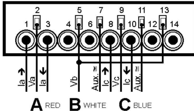
Figure 18 Two-element meter connection
