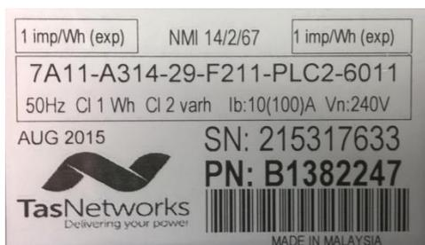
Figure 2 Example of meter faceplate showing meter number (PN) and barcode
