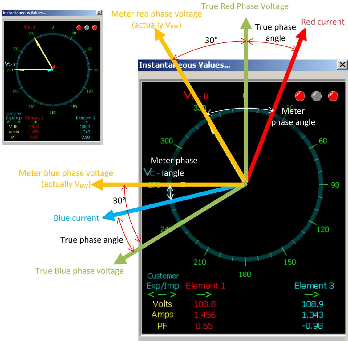
Figure 23 Two-element phasor diagram
