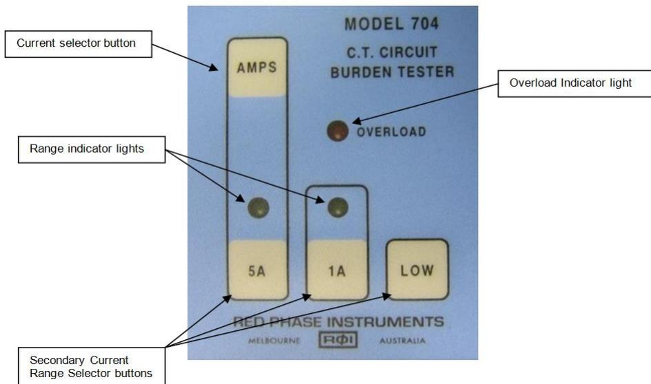
Figure I-1 Model 704 CT Circuit Burden Tester and control panel
