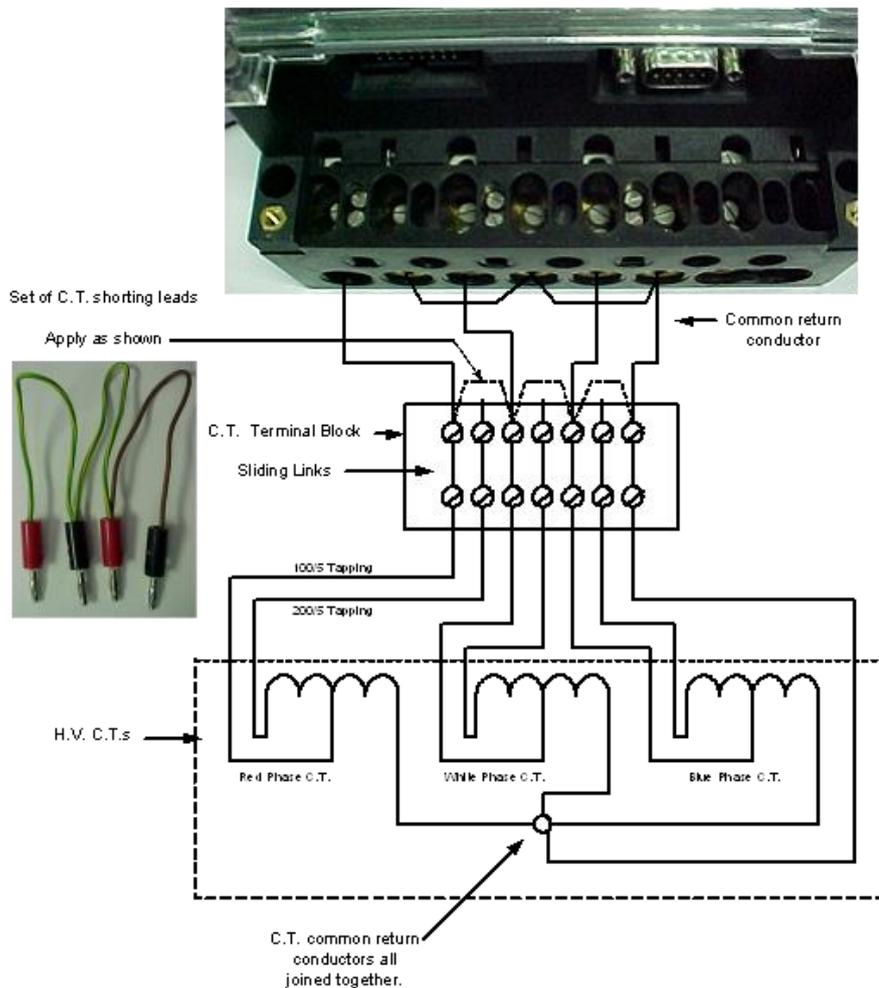
Figure 20 Three element star VT HV metering configuration with common return conductor
