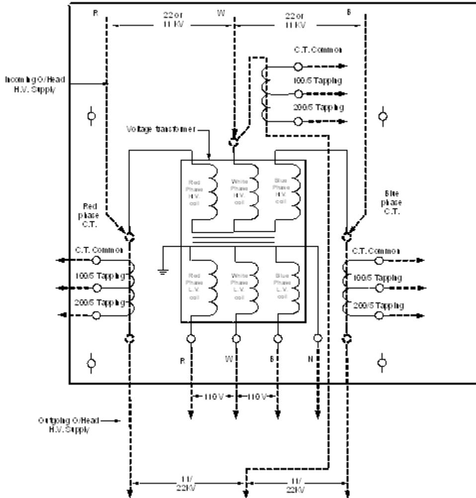
Figure 19 Three element star VT HV metering configuration
