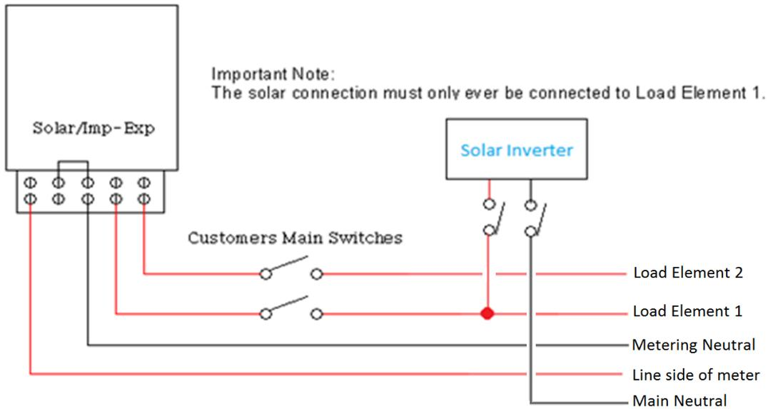
Figure 4 Wiring diagram for solar import-export meter. Note that the connection diagram above is depicting an EM1210 terminal block.
