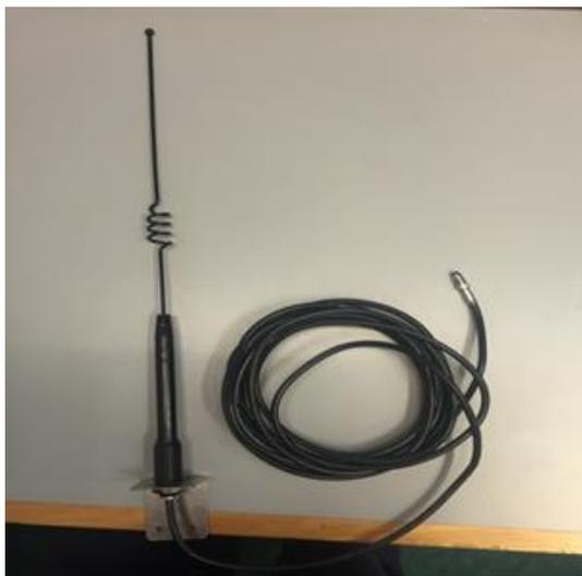
Figure 33 Standard 4.5 db gain antenna
