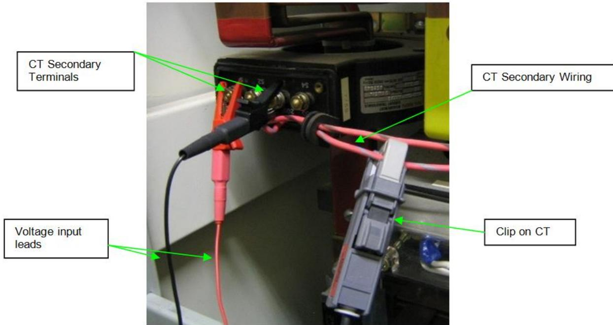
Figure I-2 Connecting the CT burden tester
