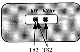
A circle surrounds each flashing dot. If a dot is flashing, it means energy is being consumed by the customer. If a circle is flashing, energy is coming from the customer or there is a connection problem.
