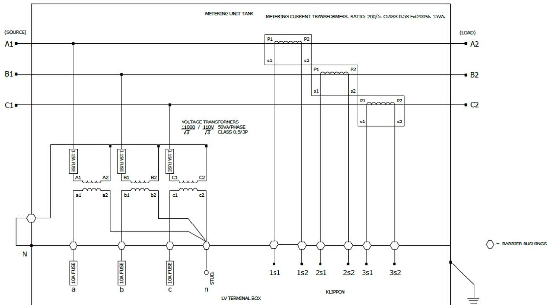
Figure 15 TWS Energy Controls HV metering unit
