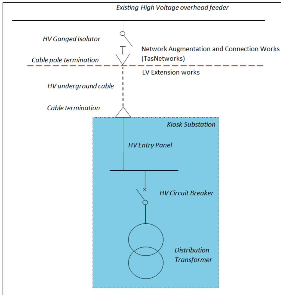
Figure 2: Kiosk connection off an existing overhead system.
