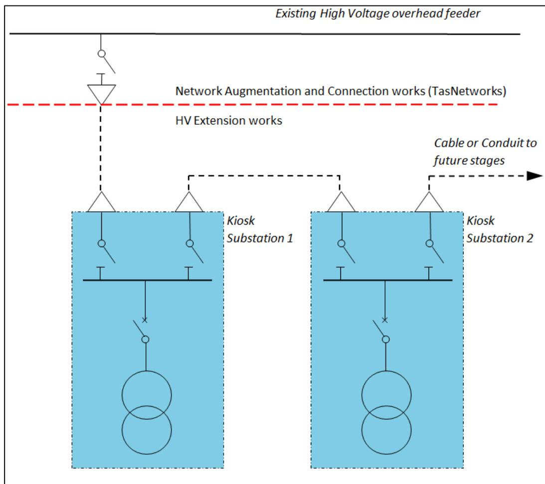
**Figure 3: Kiosk connection using a RMU for future development.**
