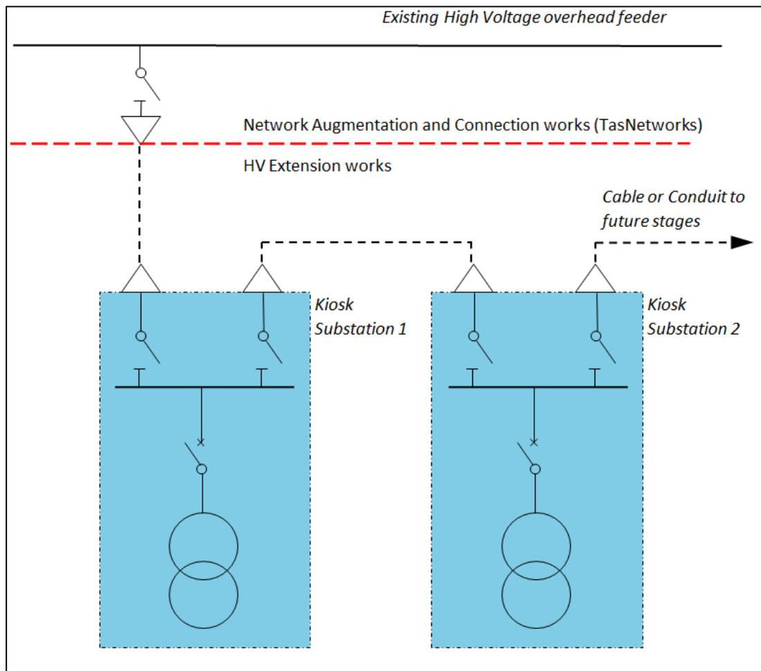
**Figure 3: Kiosk connection using a RMU for future development.**
