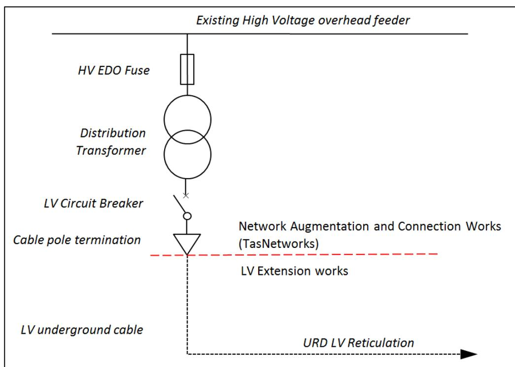
**Figure 1: LV connection from pole mounted transformer.**
