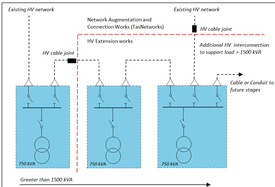
**Figure 6: HV Interconnector using a 3way HV switchboard arrangement.**
