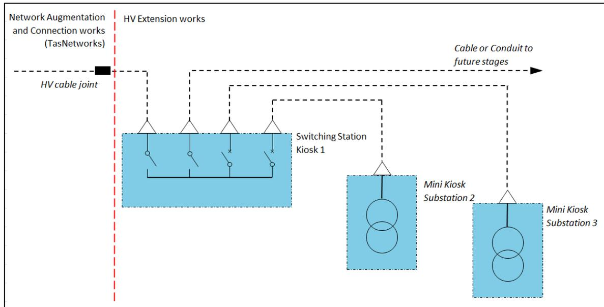
Figure 5: HV switching station with 2 remote mini kiosks.
