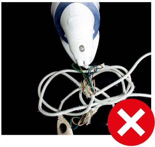
I only use electrical appliances with undamaged power cords.
