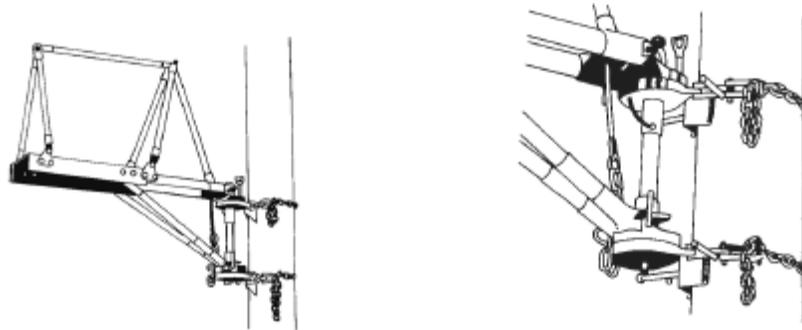
**Platform Railing** Provides an insulated horizontal rail, mounted 600 mm above the platform tread surface. This is used as the attachment point for the safety harness or body belt lanyard. (Pole strap).
