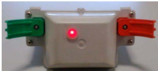
3. At the end of the test the LED will blink a number of times showing a larger flashing light to indicate the battery charge level and;
