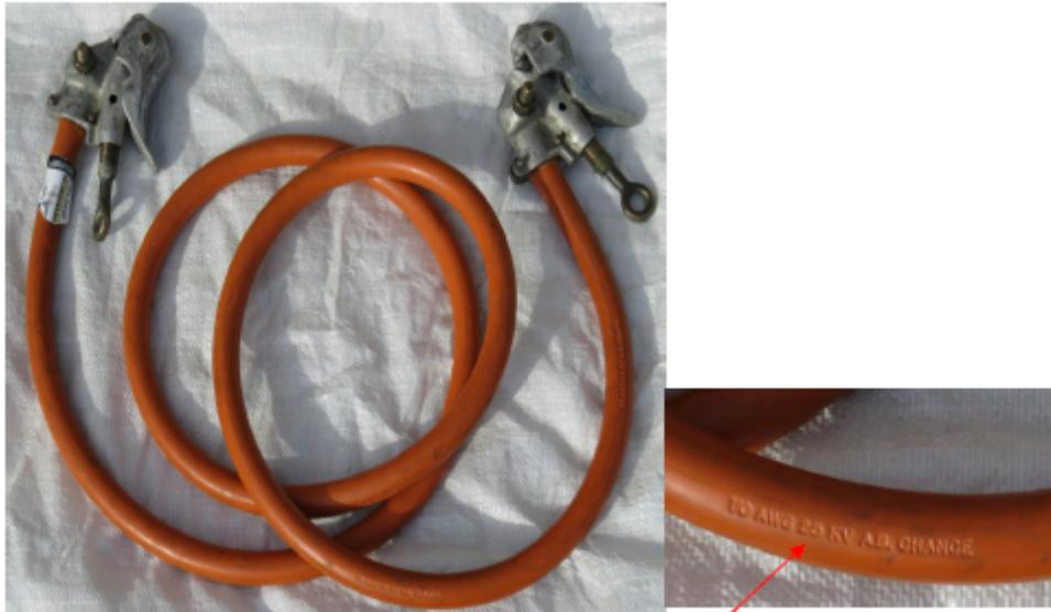
**(b) Stick Application – insulation rated to 25Kv**
