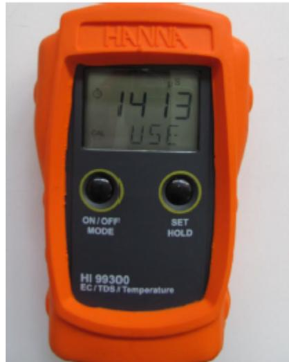
5. Place the test probe into a bottle of Calibration Solution (HI 7031 @ 1413  $\mu\text{S}/\text{cm}$ )
