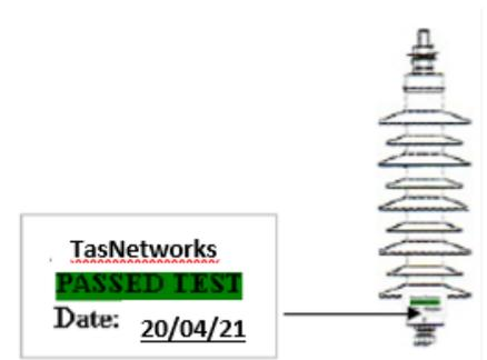
Newly tested lightning arrestors shall have a passed test sticker affixed as shown, indicating the new test date.
