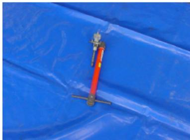
Used to support the end of temporary bypass jumpers.
