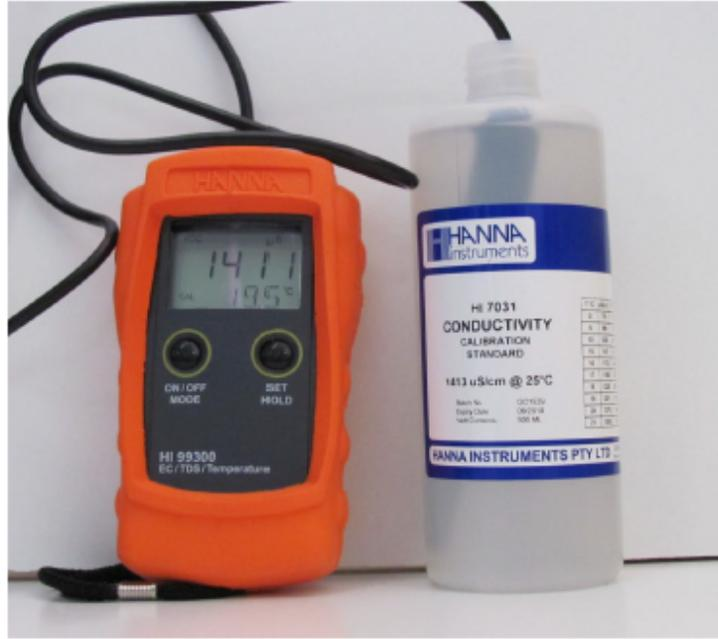
This is a method used to calibrate the HANNA Instruments HI 99300 Water Resistivity Meter. This **MUST** be performed when the Instrument display does **NOT** show the Calibration (CAL) symbol in the lower left corner of the display screen.
