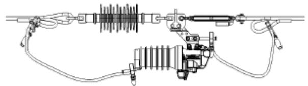
**CAUTION:** As the isolation occurs within the switch with no visible confirmation, it is necessary to disconnect and park the temporary bridge to ensure a visual break and confirmed isolation is made prior to personnel performing work on the load side of the switch.
