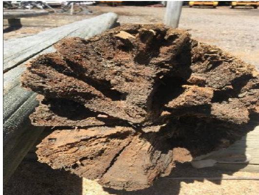
E.g. Unassisted Pole Failure
