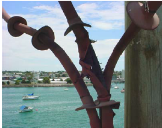
E.g. Failure of HV Cable Crutch
