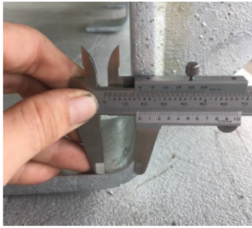
Fig 1 – Newly manufactured 32.34.58 cross arm hung transformer bracket – Larger bending radius
