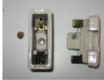
Poor rewirable fuse wedge contact
