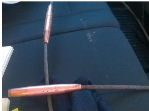
Cable pulled out of copper push pull
