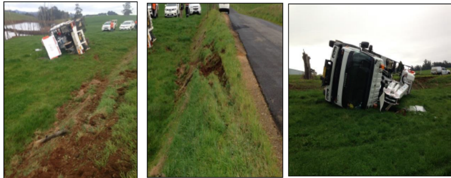
Example – soft road edge causing roll over from poor set up of EWP
